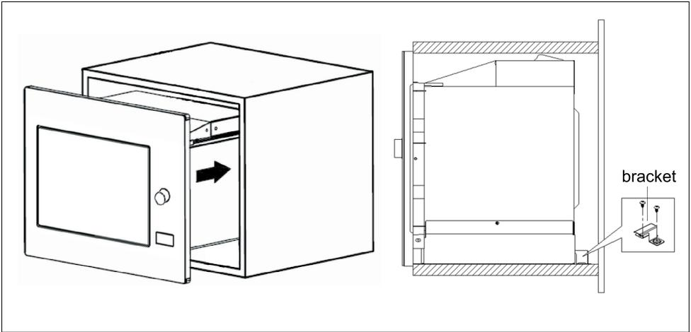
5. Open the door, fix the oven to the cabinet with Screw B, at the installation hole. Then fix the Trim-kit plastic cover to the installation hole.
