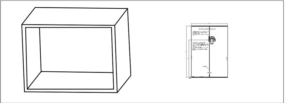
2. Make the marks on the bottom plane of cabinet according to marks "a" of of the template
