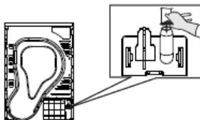
Using pliers remove the drain tube from the connector
