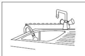
Normally condensed water drains into the container in the upper left corner of the dryer. Optionally, you can use the drain hose in the accessory bag and connect it to the dryer. Connect the hose as shown here.
